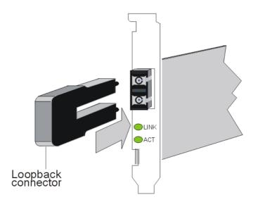
Figure 5. Setup for loopback testing
